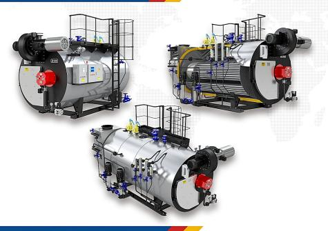
3-Pass & 3-stage energy saving Wetback design Steam capacity: 10~30t/h Working pressure: 1.25~2.5Mpa Thermal efficiency: 98% Combustion efficiency: 99.9% Feeding Water temperature: 104°C
