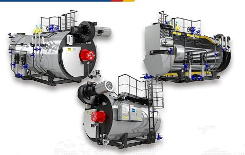
3-Pass & 2-Stage energy-saving Wetback design Steam capacity: 2~8t/h Working pressure: 1.25~2.5Mpa Thermal efficiency: 98% Combustion efficiency: 99.9% Feeding Water temperature: 20°C
